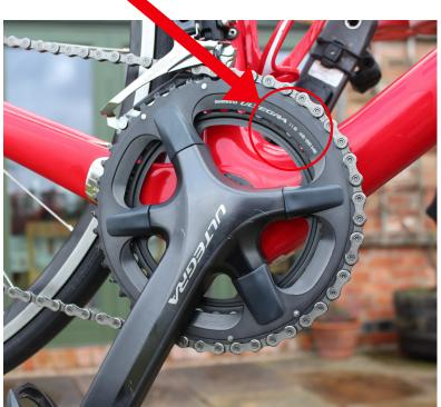
Cyclo-cross chainsets fit into the compact and/or mid-compact categories. These are a 46/36 and are produced by most of the leading brands, Shimano, SRAM, FSA. They are an excellent choice for T2\*/T3 and Youth gear limits.
