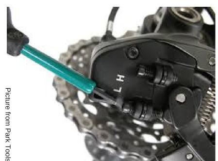
10 of it's 11 gears the problem comes when the rider clicks down into those restricted gears, which is very easy to do mid race. The limit screw will obviously block the rear mech from accessing the restricted gears, however, the servo will keep trying to access that gear and will continue to work against the limit screw. This will damage the servo and in so doing risks breaking the rear mech entirely.
